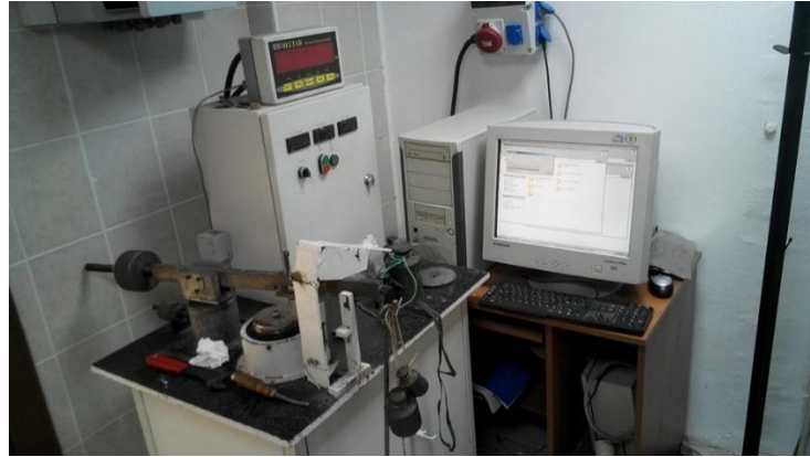
Figure 2. Pin-on-disc wear test apparatus
